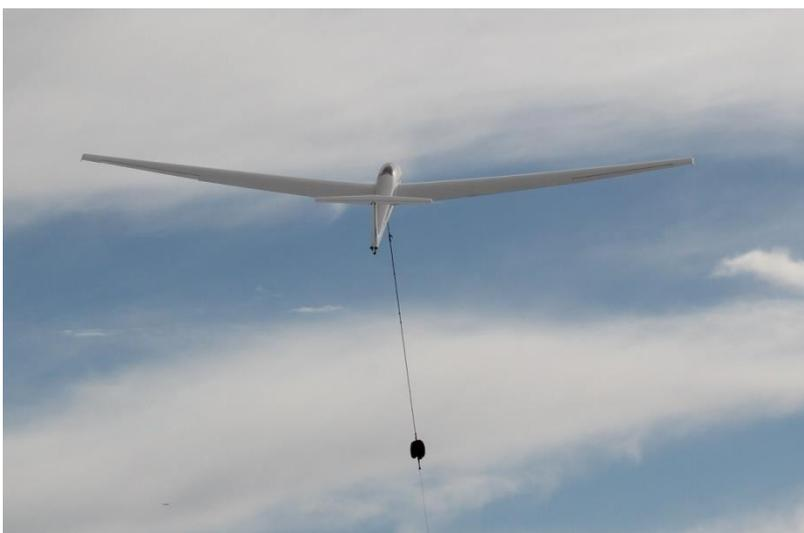
The next day we started using a winch to launch the glider. Accelerating from stationary to around 80 knots in a few seconds was amazing but I soon got used to it. We used the winch for the rest of the scholarship time and each day developed our gliding skills
