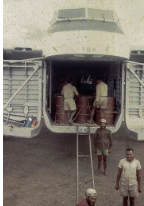
The Freighter's square hold could take a complete bulldozer, but still needed careful packing
