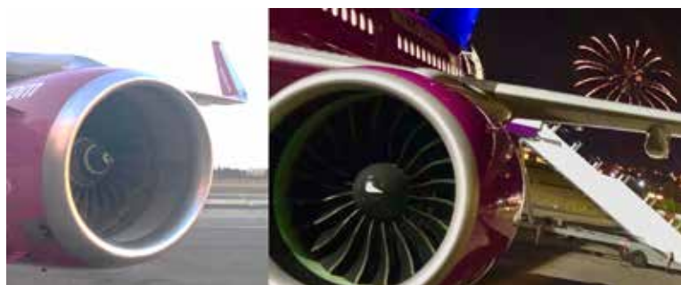
Same aircraft, greener powerplant: (Left) The International Aero Engines IAE V2500 Current Engine Option (Right) Pratt and Whitney PW1000G which produces 20-30% fewer emissions than the V2500
