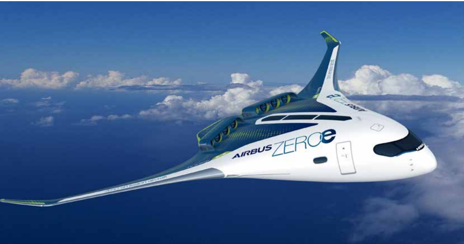
Future aircraft concepts like the Airbus ZEROe use blended wing body (BWB) airframe design and hydrogen fuel to emit zero carbon dioxide. 2035 is the earliest possible date this technology will become available (Airbus)
