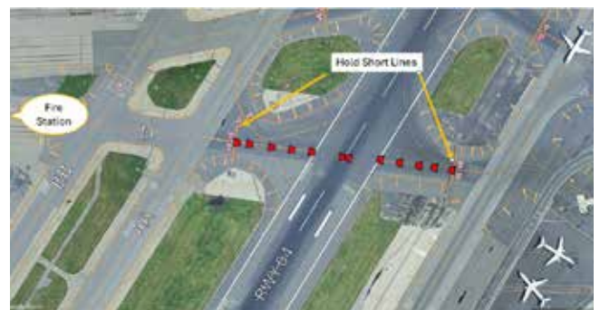
The illuminated (directional) Runway Entrance Lights protecting the intersection where the collision occurred
