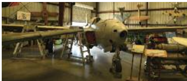
Bell YP-59A Airacomet under restoration to flying condition. (Planes of Fame)
