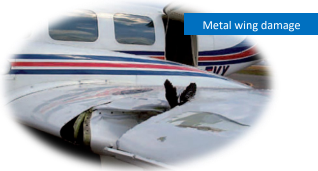
Damaged prop leading to fuselage impact
