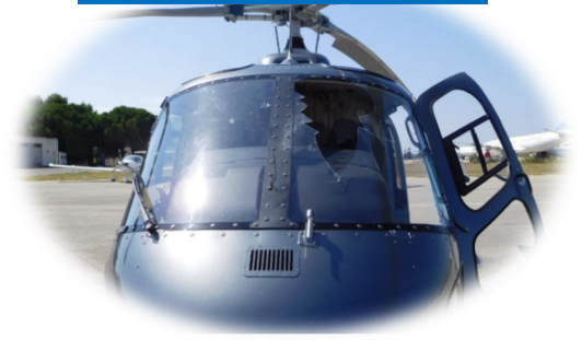
Holed helicopter windshield
