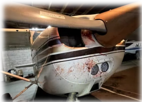
Evidence of bird impact through the propeller arc
