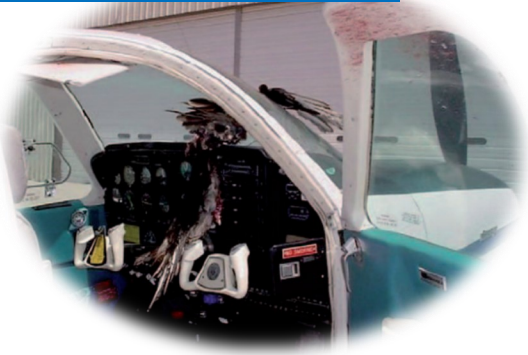
Bird carcass embedded in otherwise intact windshield
