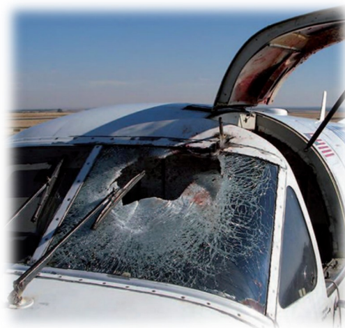
Typical windshield damage
