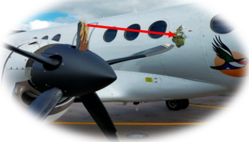
Damaged prop leading to fuselage impact
