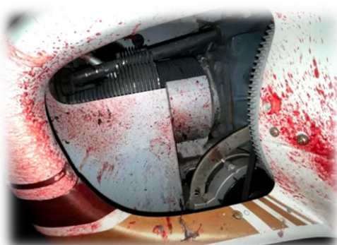
Evidence of penetration of the engine compartment
