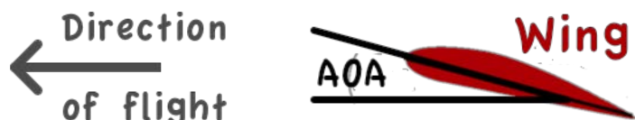
Figure 8b: Wing angle of attack (AOA)
