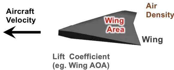
Figure 11a: Wing; Factors affecting lift
