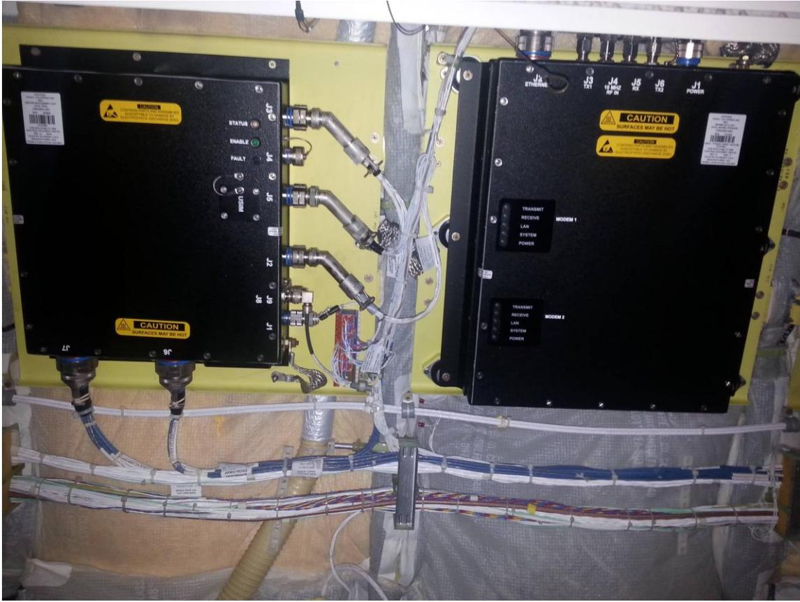
The SMU also provides the switching of data from various peripherals located in the aircraft cabin and utilizes an aircraft digital computer interface to receive aircraft position, state of flight, etc. The SMU also receives aircraft level discrete inputs to detect various conditions, including the Weight-on-Wheels signal.
