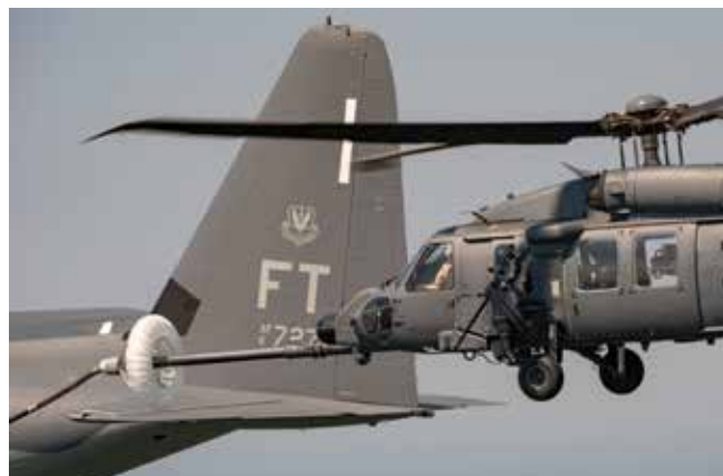
Different helicopter, same technique: a UH-60 Blackhawk clearly demonstrates the need to be above the hose of the tanking Hercules (via Author)
