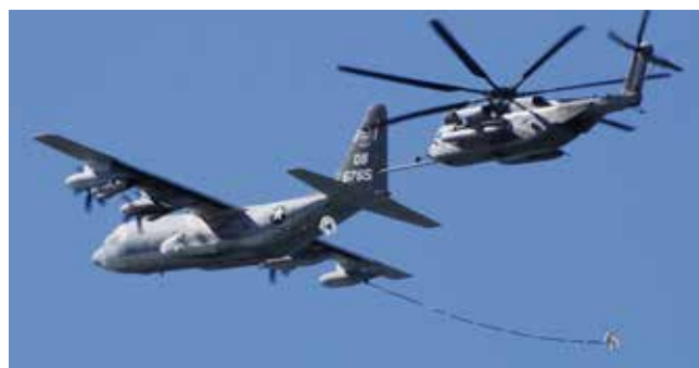
Probe extended, a Sikorsky CH-53 prepares for refuelling from a KC-130 Hercules (iStock)
