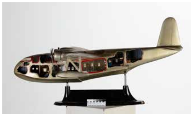
Cutaway model shows the arrangement of accommodation on the C Class
