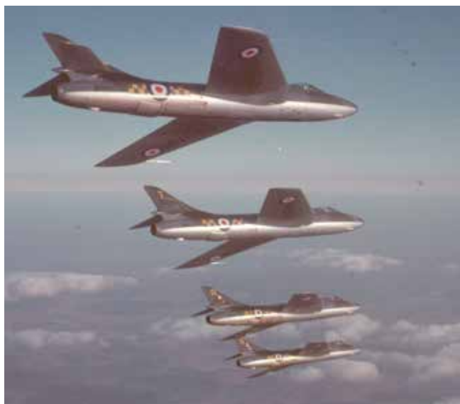
Armstrong Whitworth built 45 F.Mk.2s, fitted with Armstrong Siddeley Sapphire turbojets, of 257Sqn Wattisham, 1955.
