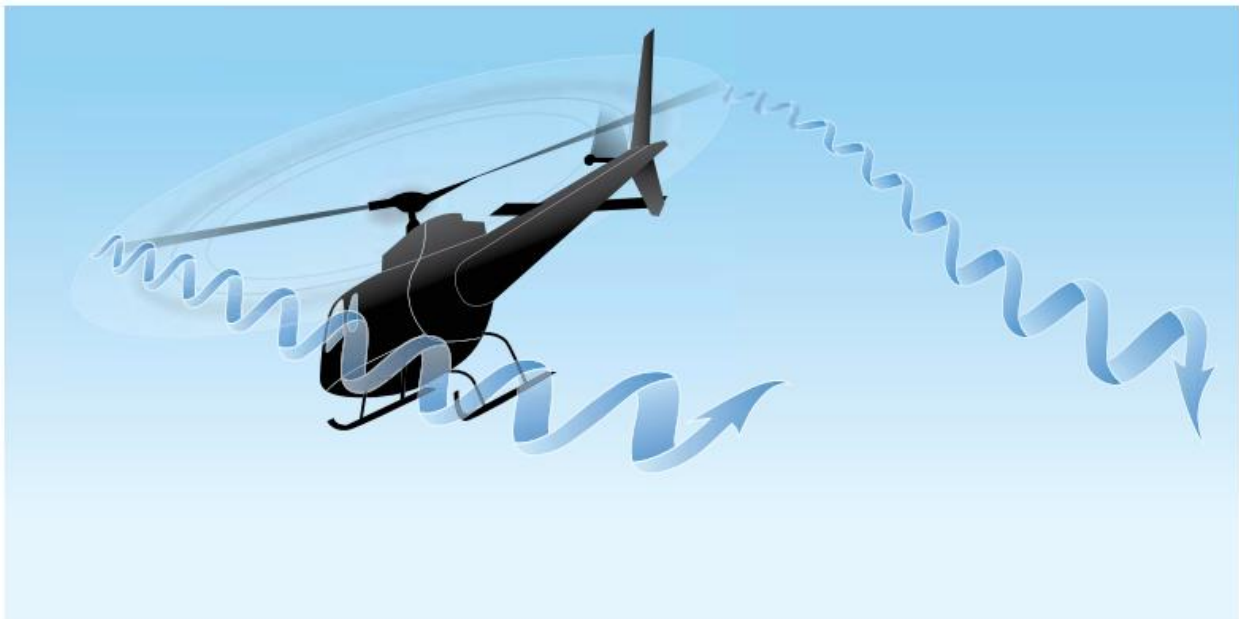
Simplified wake vortices generated from a helicopter in forward flight.
