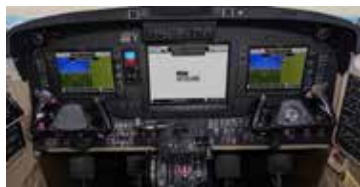
Autoland is available for aircraft such as the Beechcraft King Air 350 fitted with Garmin G1000 NXi and G3000 avionics (Garmin)
