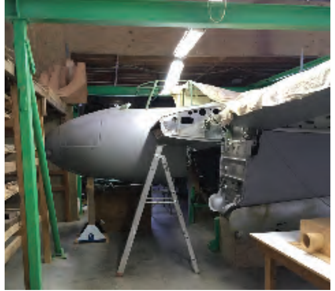
Partially completed Mosquito aircraft, Glyn Powell's workshop, near Auckland
