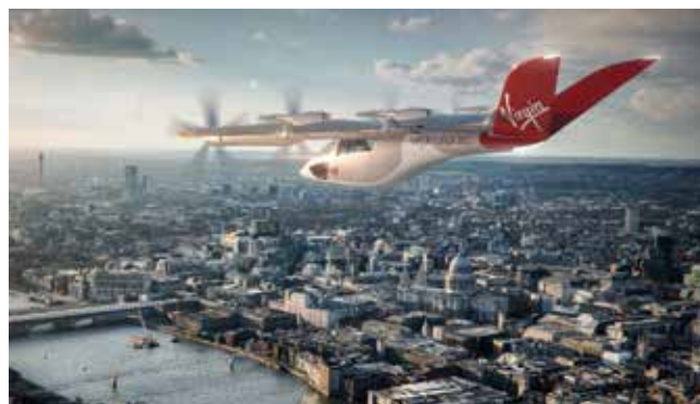
Lift-and-Cruise is seen as the most viable configuration for eVTOL – this is the Vertical VA-X4 (Vertical Aerospace/Virgin Atlantic)
