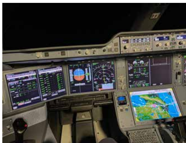
The A350's ACMS gives vital information during the test flight
