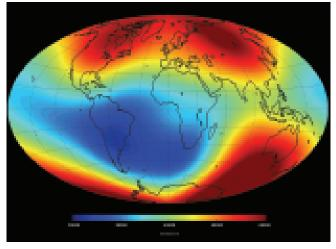
Map 2 shows memory upsets from the stalwart British satellite UOSAT-2 which broadcast telemetry for over thirty years, from 1984 to 2015
