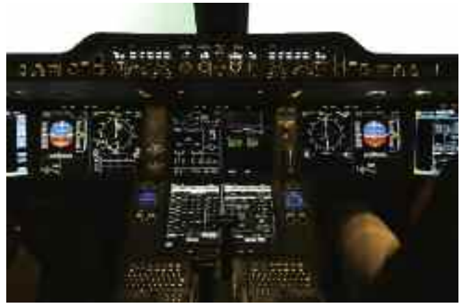
The flight deck of an A350-900 on approach into Bordeaux, France. The artificial horizons and compass indicators are visible at both pilot positions (McCullins).
